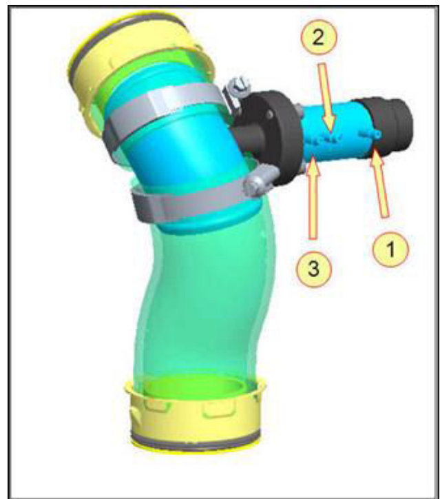
Figure 2: Vacuum hose routing on temperature switch, showing ventilation hose to air cleaner (1), hose to vacuum source (2), and hose to charge air cooler regulator flap (3).
