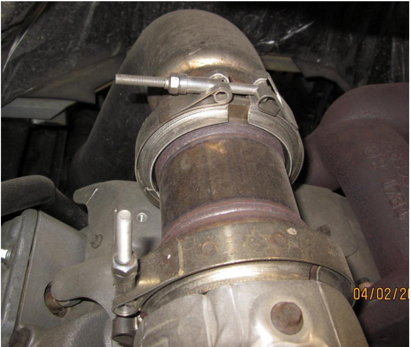
Install Gasket between two Flanges
