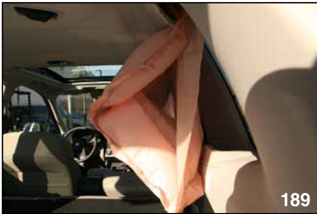
CURTAIN AIRBAG DEPLOYED VIEW FROM BACK OF CAR
