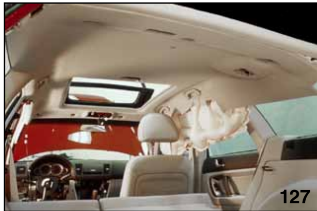
CURTAIN AIRBAG DEPLOYED
