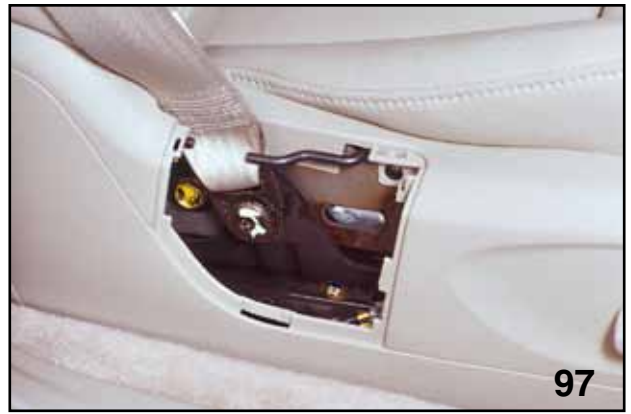
SEAT BELT ANCHOR COVER REMOVED
