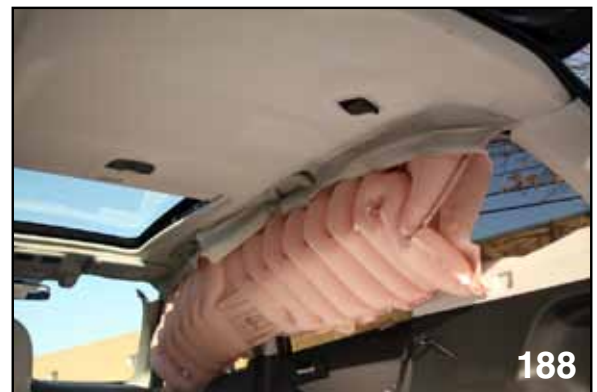
HEADLINER AFTER CURTAIN AIRBAG DEPLOYED
