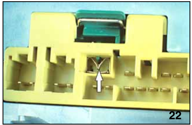
PRIMARY DOUBLE LOCK CONNECTOR (UNLOCKED)
