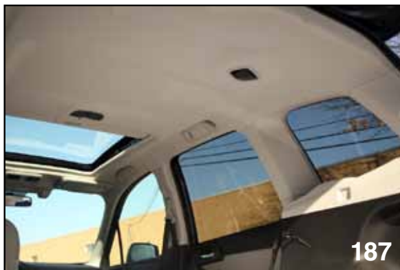
HEADLINER BEFORE CURTAIN AIRBAG DEPLOYED
