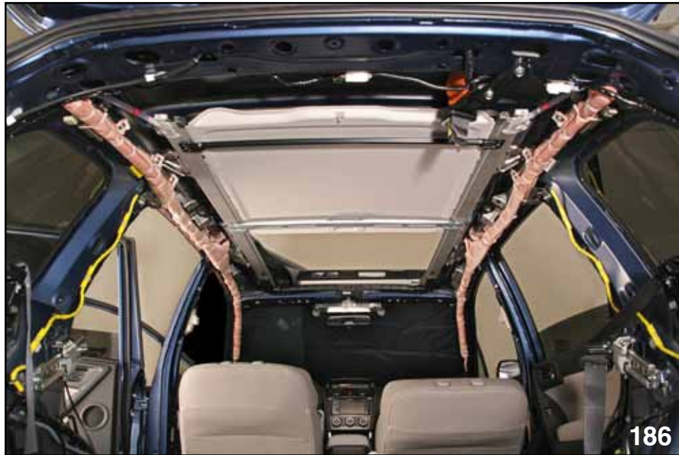
CURTAIN AIRBAG MOUNTING
