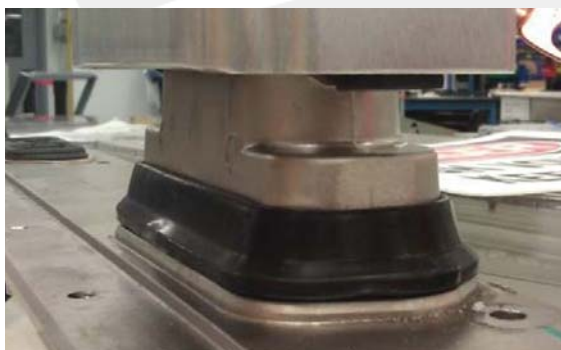
Figure 16: Inner seal not fully engaged
