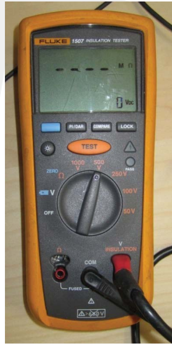
Figure 4 (Fluke 1587, set to 500V, positive lead connected to insulation jack)
