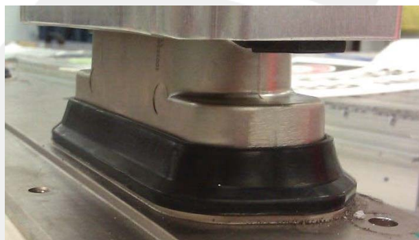
Figure 17: Inner seal fully engaged
