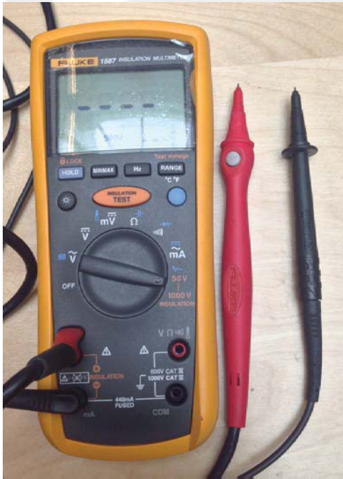
Figure 3 (Fluke 1507, set to 500V, positive lead connected to insulation jack)
