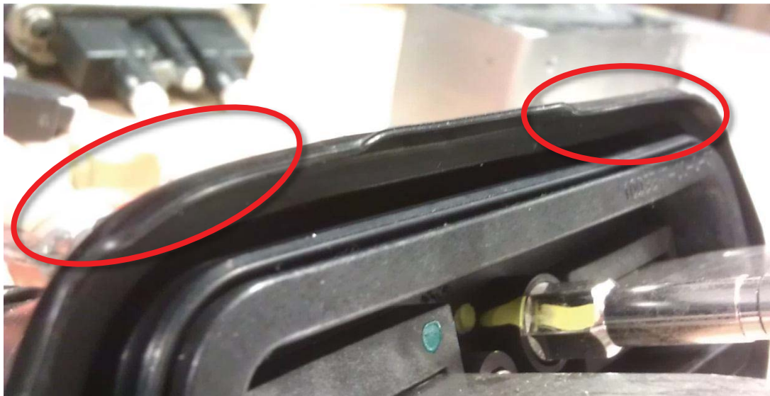
Figure 5 (Seal deformed inwards)
