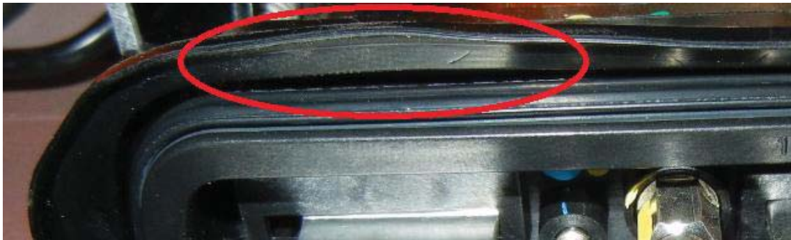
Figure 4 (Seal deformed outwards)
