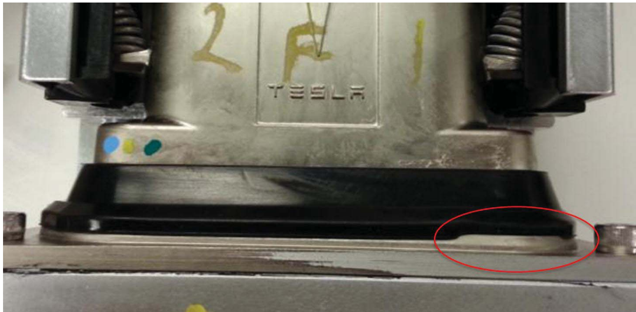
✗ Incorrect – Skirt seal caught on base Figure 18
