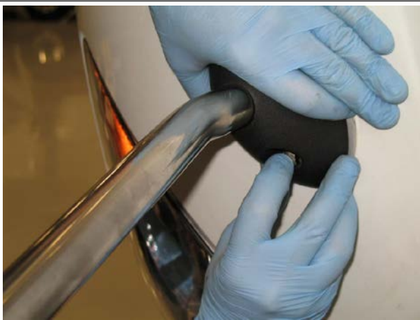
Figure 14. Single-Bolt Stanchion Installation.
