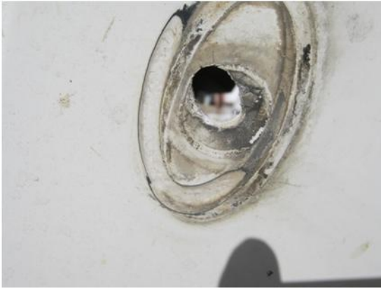
Figure 1. Existing Wear to Production Hood-Mounted Mirror System.
