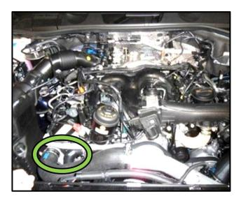
Section B - Install Spacer ring
