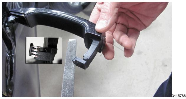
If the thickness is between 5.7 mm (0.224 in) and 5.9 mm (0.232 in), the door handle leg does NOT require modification. Proceed to step 8.
