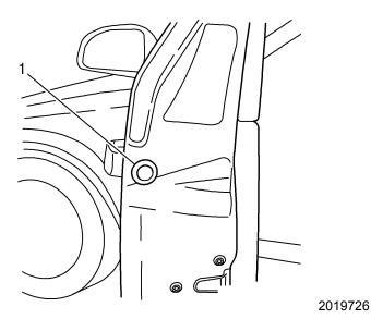
11. Install the cover cap that conceals the screw (1) to the inside edge of the door.
