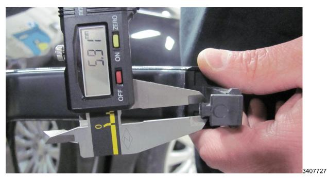
7. Measure the leg of the door handle as shown. Ensure the thickness is between 5.7 mm (0.224 in) and 5.9 mm (0.232 in).
