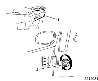
**Note:** Handle will snap back to flush condition. Turn the fastener in the clockwise (right) direction until proper torque is reached.
