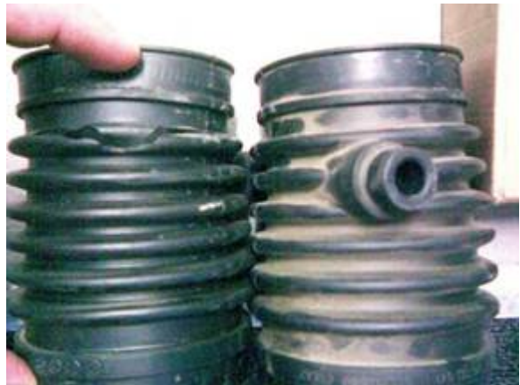
Figure 3. Crack in the intake hose.
