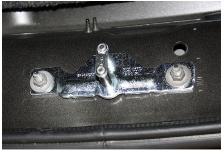
Figure 5. Manual lid style striker plate studded mounting.
