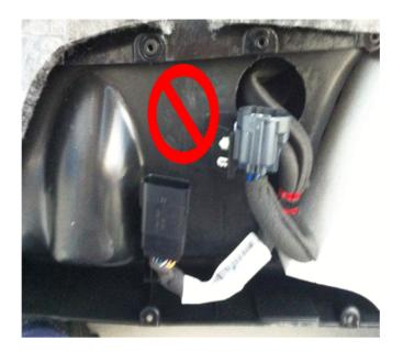
**Important:** The correct harness routing is shown in the first graphic above. An example of an incorrect routing is shown in the second graphic.
