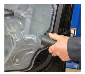
6. For a higher level of assurance of a complete seal of the deflector to the door surface, using a hand held roller or similar tool, "wet-out" the butyl adhesive around the complete perimeter of the water deflector.
