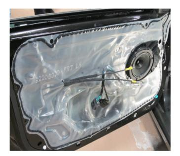
1. If a side door leak is verified, remove the trim panel on the affected door. Refer to Front or Rear Side Door Trim Panel Replacement in SI.
