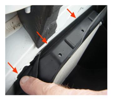
2. Inspect the seam at the top of the HVAC case, where the case sits against the cowl. The seam is commonly not sealed in this area and water coming off the windshield may find a path behind the case and leak into several places in the interior under the dash.
