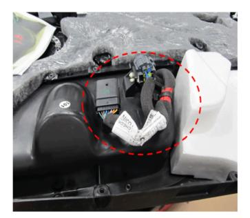
8. If repairing a leak at the driver door, inspect the routing of the mirror and window switch harnesses before installing the trim panel:
