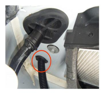
• For some police equipped vehicles, water may run on the wire harness exiting the HVAC case, then follow along the conduit into a grommet/hole (shown circled in the graphic above) in the cowl, and finally run into the vehicle interior.
