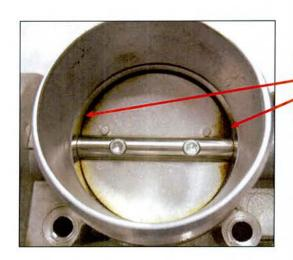
Heavy deposits at the valve to the bore interface.
