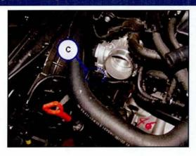
Remove the 4 ETC throttle body mounting bolts and then pull out the ETC throttle body away from the intake manifold.
