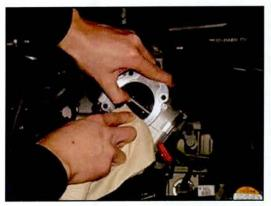
5. Reinstall all the removed parts in reverse order of removal after completing the ETC throttle body cleaning.
