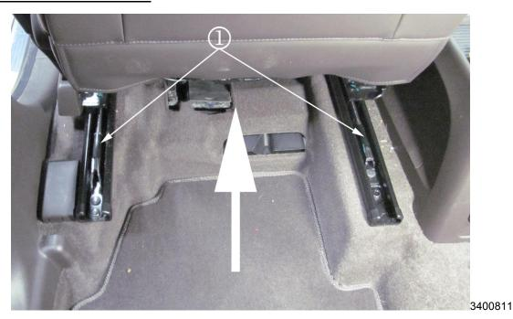
1. Adjust the driver seat to the full forward position.
