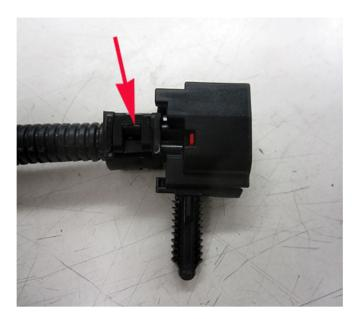
4. Remove the connector to conduit collar.
