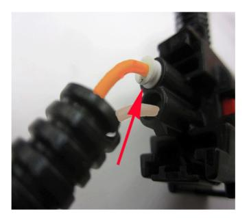
• If the wire is not fully seated, replace the connector.
