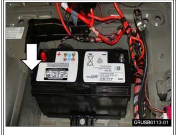
Important Note: Before mounting the battery in place, make sure the battery vent hose is connected as indicated by the arrow.
