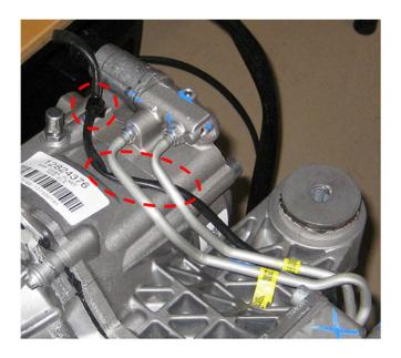
21. Reinstall the electrical connector to the limited slip differential valve and harness to the clip. Route the electrical harness under the pressure lines as shown.
