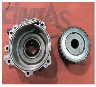
10. Remove the differential clutch pack from the clutch housing. Hold the housing in one hand and flip over to allow the clutch pack to fall into the other hand.
