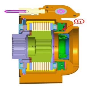
3. If the rear differential fluid level is too high and either a or b exists, then the eLSD clutch oil is leaking past the eLSD clutch internal piston seals (6 or 7) into the rear differential. The service fix is to replace the eLSD clutch piston only using the following procedure.
