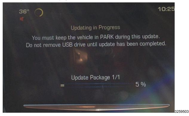
8. Once Update has been selected from the display, the screen in the picture above will appear. This screen will show the progress of the update. The navigation software update will take about 2 hours to load. The non-navigation software will take about 30 minutes to load.
