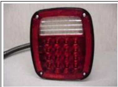
Truck-Lite Tail Light Includes Integrated Pigtail
