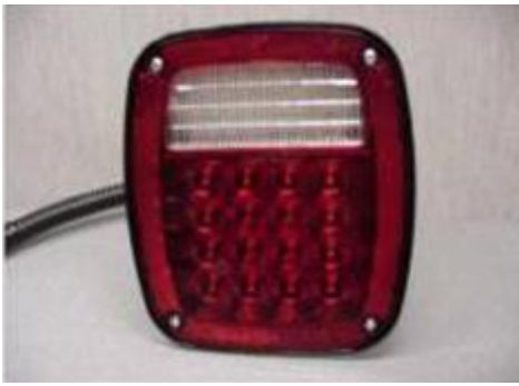
Truck-Lite Tail Light Includes Integrated Pigtail
