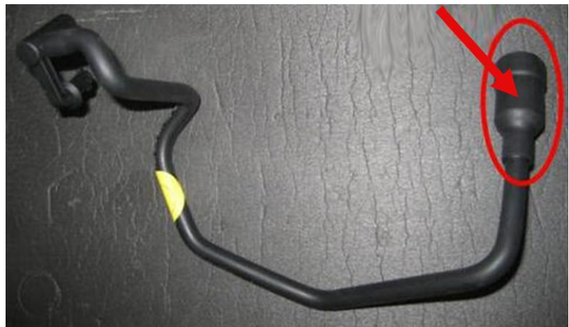
Figure 2. Updated ventilation hose with integrated filter.
