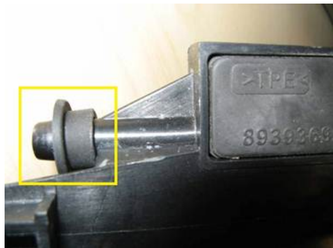
Figure 5. Ring seal installed on headlamp air tube.
