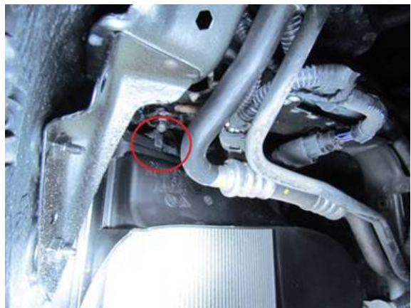
Figure 10. View of exit air duct affixed to mounting hook.
