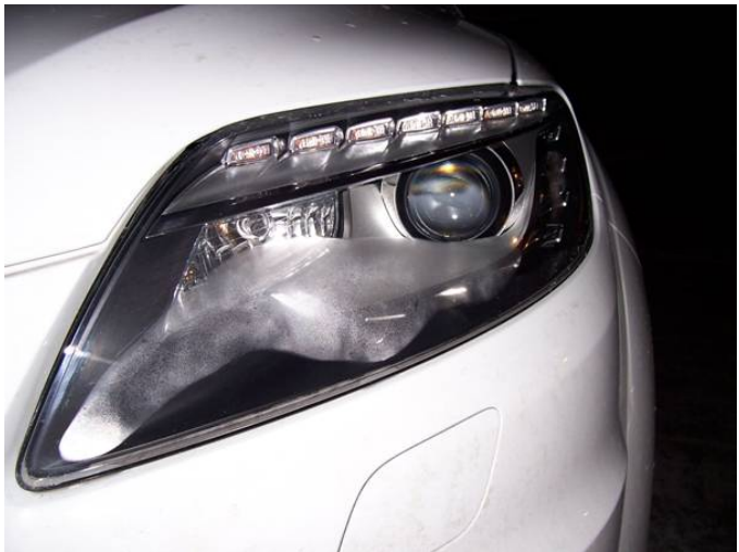
Figure 1. Moisture in headlamp.
