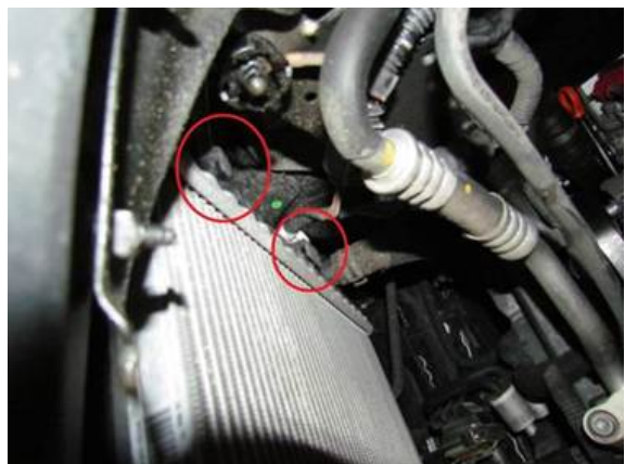
Figure 8. Upper exit air duct attachment points to charge a cooler.
