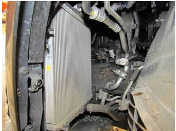
Figure 6. View of charge air cooler with wheel well liner removed.
