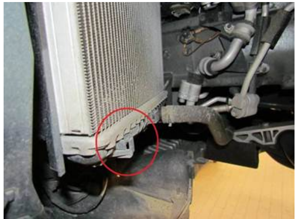
Figure 7. Lower exit air duct attachment point to charge air cooler.
