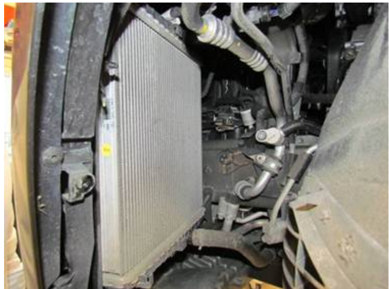
Figure 9. View of charge air cooler with wheel well liner removed.
