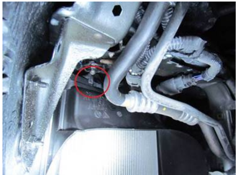
Figure 13. View of exit air duct affixed to mounting hook.
