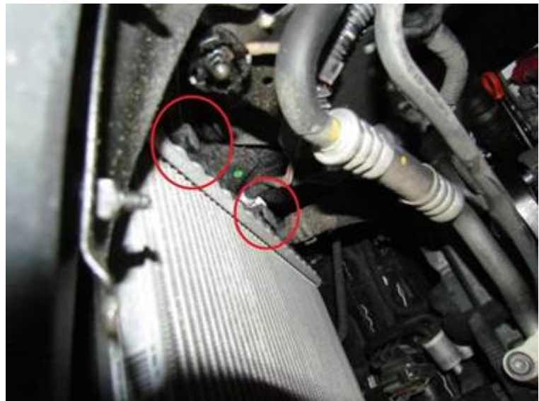
Figure 11. Upper exit air duct attachment points to charge a cooler.
