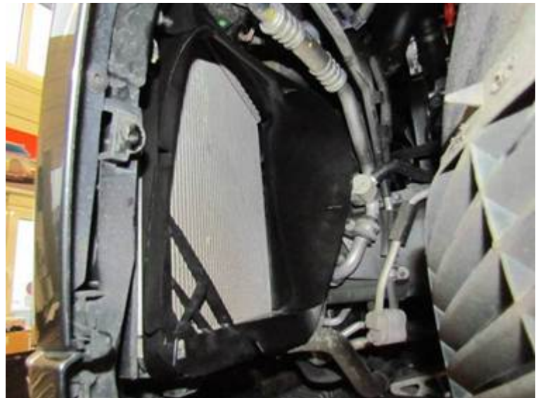
Figure 12. Charge air cooler exit air duct installed.
