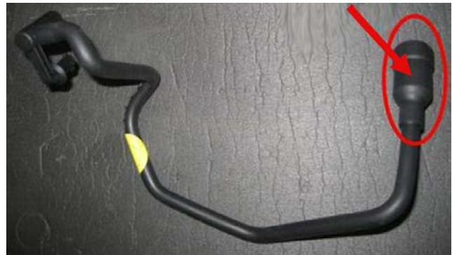
Figure 2. Updated ventilation hose with integrated filter.
