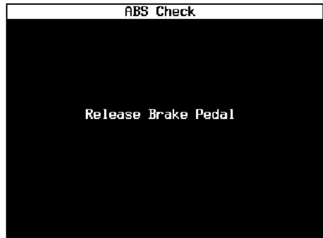
19. If all the wheel circuits (left front, right front, left rear, and right rear) have passed the check, the ABS Hydraulic Modulator is good. Continue to the Brake Valve Cycling section of this bulletin (**SECTION "B" beginning on page 11**) to complete this recall.
