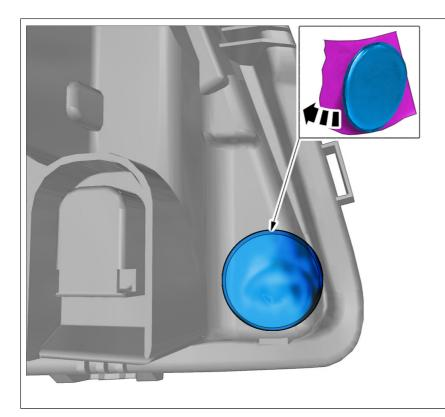
Note! Ensure that the tape is fixed to the surface.
