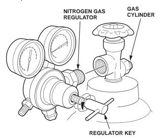
3. Connect the high pressure hose from the kit to the solenoid valve adapter and the gas regulator. Make sure the nitrogen tank is supported safely.
