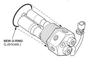
Hand thread the solenoid valve into the tank making sure the O-ring seats properly into its groove.
