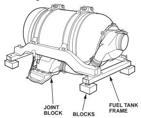
Use the large plastic wire tie to support the fuel joint block lines up to the frame. Make sure that the joint block bracket is attached. Leave the wire tie in place until the lines are reattached to the new solenoid valve.
