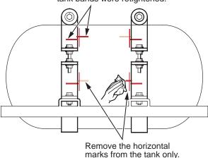
12. Re-mark the fuel tank horizontal lines using the yellow paint marker supplied in the kit. Trace over the original lines that remain on the tank bands, and paint the lines about 1.5 to 2 inches long on the tank. It is important to mark accurate lines, as these new lines will be used to evaluate proper tank positioning. The lines you paint may go over the label, but this is not a concern.
