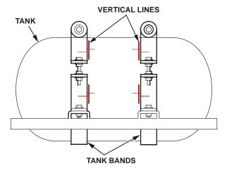
10. Install and torque the spring retaining bolt lock nuts to 38 N•m (28 lb-ft).
