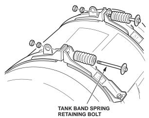
4. With the help of another technician, carefully rotate the tank assembly as needed until the three fuel line flanges align flush with the line connector position (hold the nut back to see).
