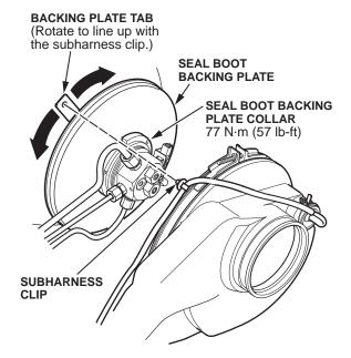
2. Tighten the seal boot backing plate collar, using the spanner from the kit, to **77 N•m (57 lb-ft)**.
