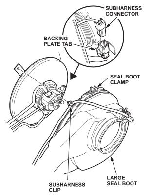
4. Connect the 2-pin solenoid sub harness connector to the wire harness on the tab.
