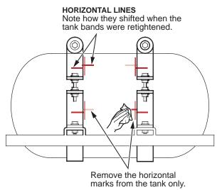
12. Re-mark the fuel tank horizontal lines using the yellow paint marker supplied in the kit. Trace over the original lines that remain on the tank bands, and paint the lines about 1.5 to 2 inches long on the tank. It is important to mark accurate lines, as these new lines will be used to evaluate proper tank positioning. The lines you paint may go over the label, but this is not a concern.
