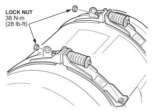
11. Remove the old horizontal paint markings from the tank only, (not from the tank bands) using contact brake cleaner.
