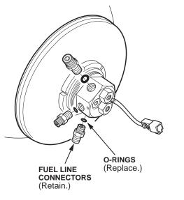
6. Note the position of the line connectors. Remove the three fuel line connectors.
