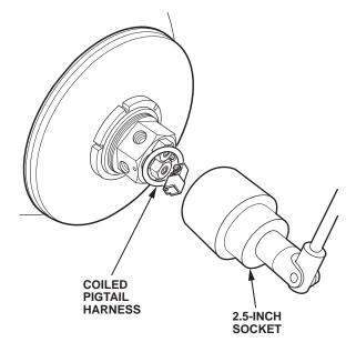
8. Use the breaker bar supplied in the kit to loosen the solenoid valve.
