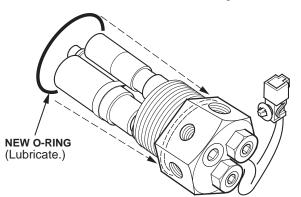
3. Hand thread the solenoid valve into the tank making sure the O-ring seats properly into its groove.
