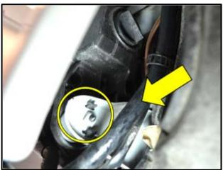
Tip: Inside the left front fender, reposition the headlight washer hose <arrow> so it rests in front of the headlamp mounting bracket <circle>. This will provide adequate slack in the hose when removing the fascia from the vehicle and prevent damage to the washer fluid line and/or fittings.
