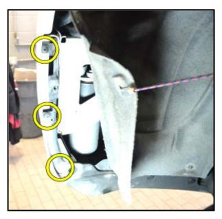
Remove the three fasteners from the fascia mounting bracket <circles>.
