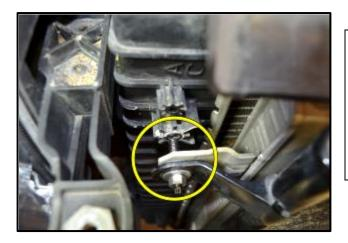
Gently pull the charge air cooler and A/C condenser forward, away from the radiator.
