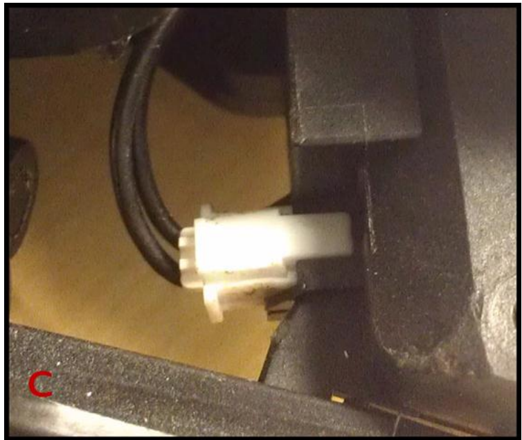
Figure 4. Connector “C” shown in the locked position.
