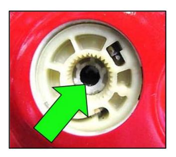
Place another large drop of adhesive part number (D 195 800 A1) as shown <arrow> into the lower corner of the regulator bore.
