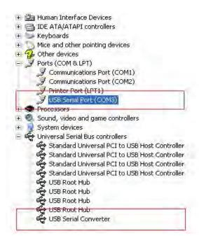
4. Once you have found the COM Port that the USB Serial Converter was assigned, you can change the setting by clicking the "Com Port Configuration Button" shown below.
