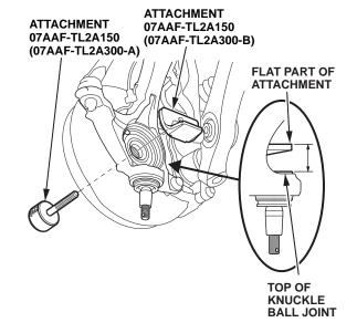
29. Position the ball joint tool kit, the adapter G, and the C-frame OTC7248 (commercially available) on to the knuckle ball joint.
