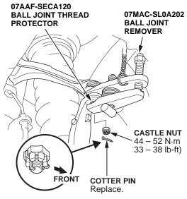
14. Disconnect the upper arm ball joint from the knuckle using the ball joint thread protector and the ball joint remover.
