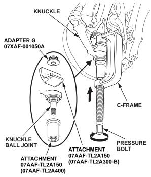
30. Tighten the pressure bolt of the C-frame, and remove the knuckle ball joint.
