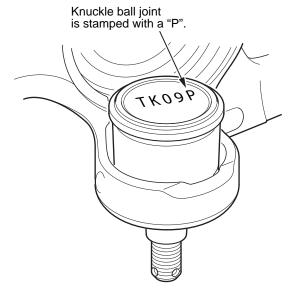
33. Position the ball joint tool kit and the C-frame, OTC7248, (commercially available) to the ball joint. Tighten the pressure bolt of the C-frame until the knuckle ball joint shoulder is fully seated in the knuckle.
