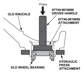
21. Press a new wheel bearing into the new knuckle using the old bearing, a steel plate, the attachment, the support base, and a press.
