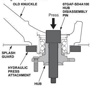
18. Press out the wheel bearing inner race of the hub using the hub dis/assembly pin, a commercially available bearing separator, and a hydraulic press.
