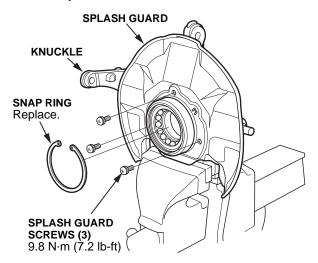
25. Install the hub onto the new knuckle assembly using the driver handle, the attachment, the support base, and a hydraulic press. Be careful not to damage the splash guard.
