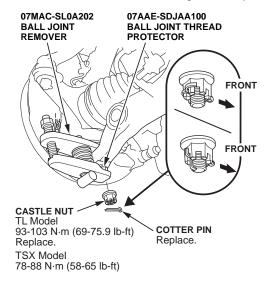
Disconnect the knuckle ball joint from the lower arm using the ball joint thread protector and ball joint remover.
