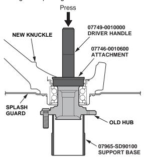
26. Install the new knuckle assembly, then go to step 35.
