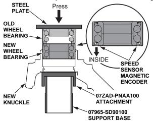
22. Set the new knuckle assembly in a vice to hold it securely and install the front knuckle ring:
