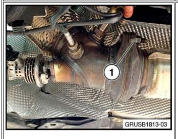
The barrel of the E90 mixer points toward the rear of the car. This is identified by the mixer tabs wrapped around the flange on the SCR cat (1).
