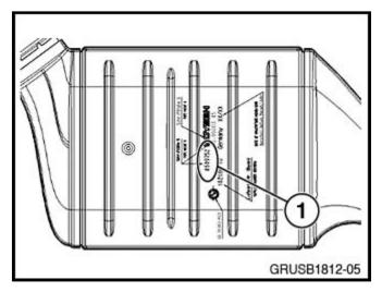
Check the part number of the SCR catalyst (1). If the part number is not 18 30 8 509 752/753 (E70) or 18 30 8 509 749/750 (E90), the SCR catalyst will need to be replaced.
