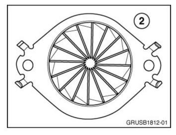
If the updated mixer has already been installed, it will have one set of fins (2). No replacement is necessary. Reinstall the SCR front pipe to the down pipe of the DPF.
