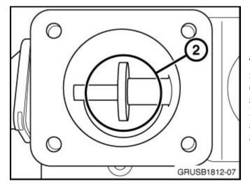
The original EGR valve has a diffuser in the airstream flow from the throttle (2). The valve for EGR actuation is seated further into the EGR airstream. Replace this valve with P/N 11 71 8 512 526 (Repair Instruction 11 71 501).
