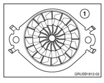
fin arrangement (1). This mixer will need to be replaced with P/N 18 30 8 513 445 (E70) or P/N 18 30 8 512 438 (E90).
