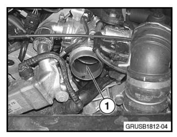
Remove the charge air pipe at the throttle (ignition off). Using a flashlight, look through the throttle (1) and inspect the EGR valve.
