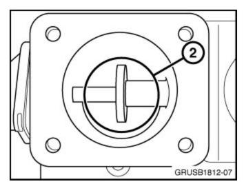
The original EGR valve has a diffuser in the airstream flow from the throttle (2). The valve for EGR actuation is seated further into the EGR airstream. Replace this valve with P/N 11 71 8 512 526 (Repair Instruction 11 71 501).
