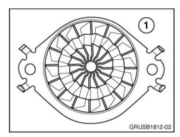
The original style mixer has a multiple fin arrangement (1). This mixer will need to be replaced with P/N 18 30 8 513 445 (F70) or P/N
