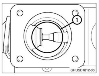
The updated EGR valve (P/N 11 71 8 517 217 or P/N 11 71 8 512 526) has the valve and seat directly in the airstream of the throttle (1). If this valve is installed, no further action is needed. Reinstall the charge air pipe.
