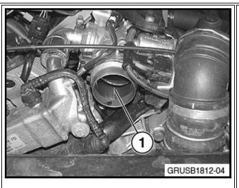
Remove the charge air pipe at the throttle housing (ignition off). Using a flashlight, look through the throttle (1) and inspect the EGR valve.
