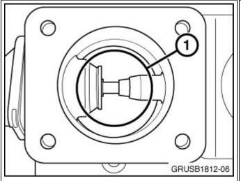
The updated EGR valve (P/N 11 71 8 517 217 or P/N 11 71 8 512 526) has the valve and seat directly in the airstream of the throttle (1). If this valve is installed, no further action is needed. Reinstall the charge air pipe.
