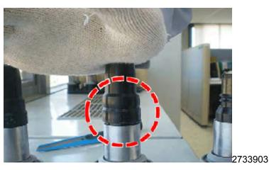
8. Insert the new boot onto the ignition coil tower fully.
