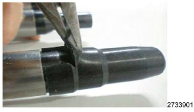
6. Remove the boot using long-nose pliers as shown in the illustration.
