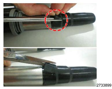
5. Using a scissors, cut bottom of boot as shown in the illustration.
