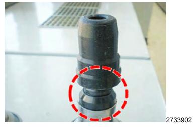
7. Insert new boot onto the ignition coil tower partially.
