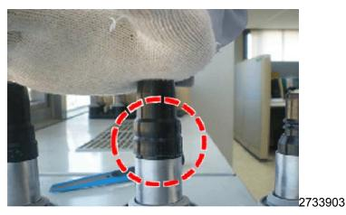
Insert the new boots onto the ignition coil towers fully. The new boot is fully seated when it is within 1 mm (0.040 inch) of metal shield.
