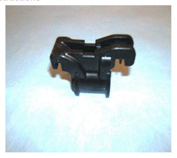
A clip has been made available to eliminate the lateral seat movement. Use the following steps to install the clip to the driver side seat. If the vehicle is equipped with a 6-way adjustable passenger seat, repeat the procedure on the passenger seat.
