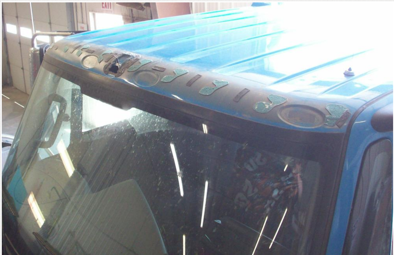
The sunshade mounting bracket has completely detached from the vehicle.
