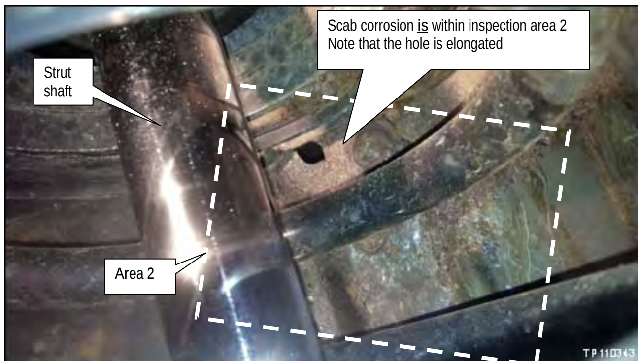
Example (Additional Photo) of Area 2 Scab Corrosion Inspection
