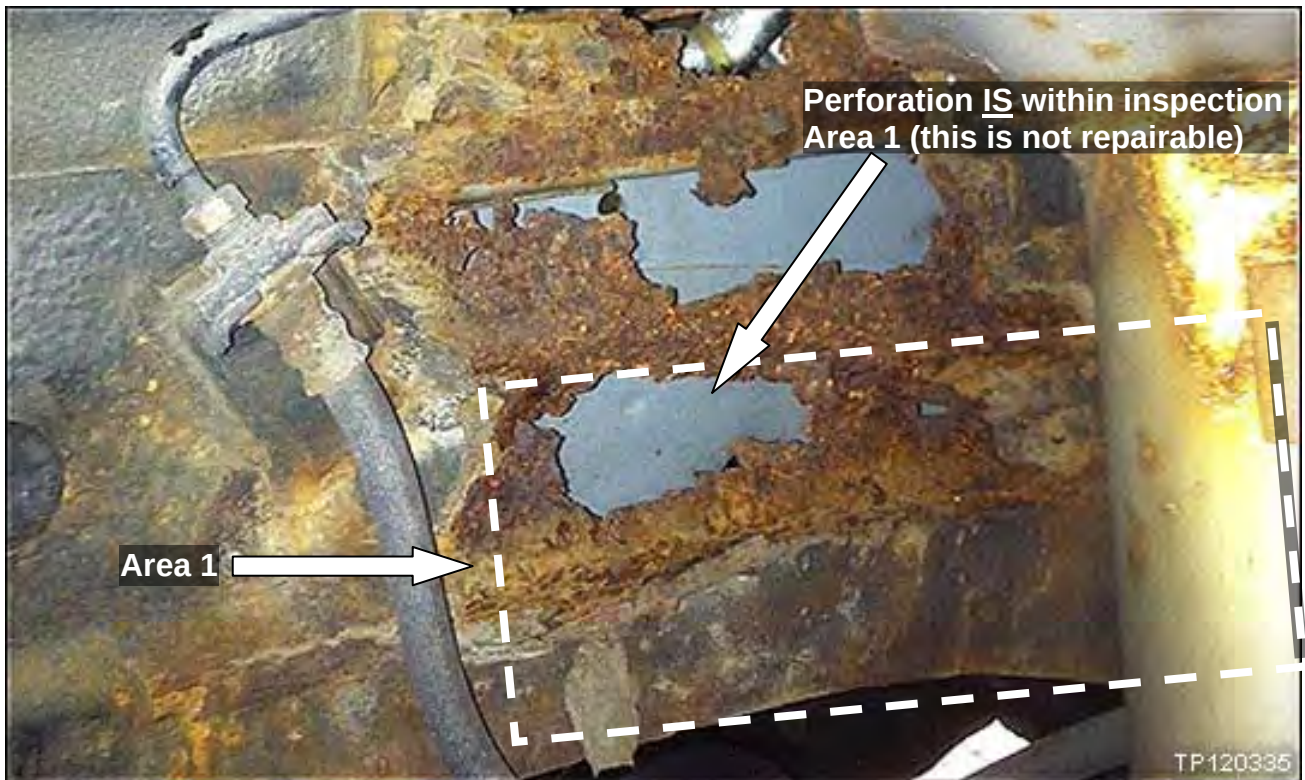
Example (Additional Photo) of Area 1 Perforation Inspection
