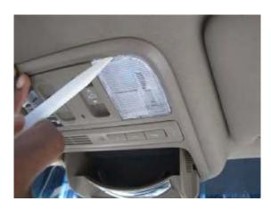
Remove the four screws from the roof console, then remove the console from the roof. You don't need to disconnect the wire harness connectors; just let the console hang.
