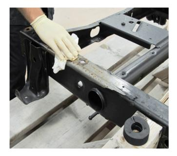
8. Using Lloyd's Pure Prep™ Metal Surface Preparation P/N 25418 (10 fluid ounce bottle), or equivalent, saturate a towel or Scotch-Brite™ (3M) pad with the pre-diluted solution and scrub the area well, rendering a foaming of the Pure Prep.™ This will greatly improve adhesion and corrosion resistance in the repair areas.
