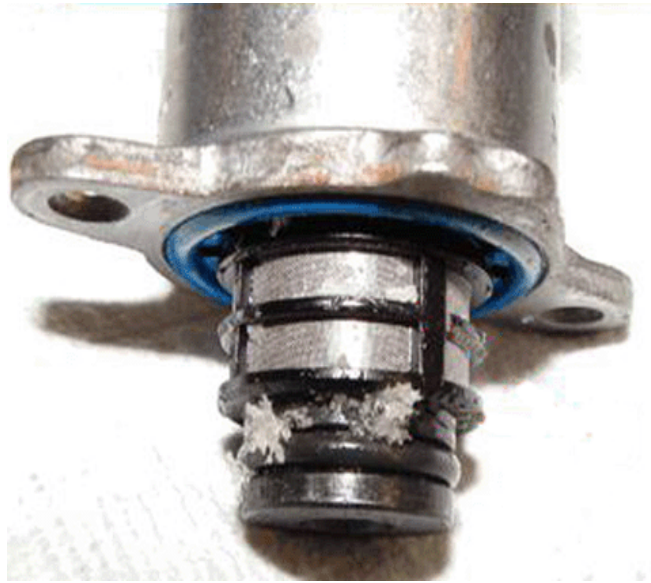
Fuel Pressure Regulator 1 Contaminated With DEF
