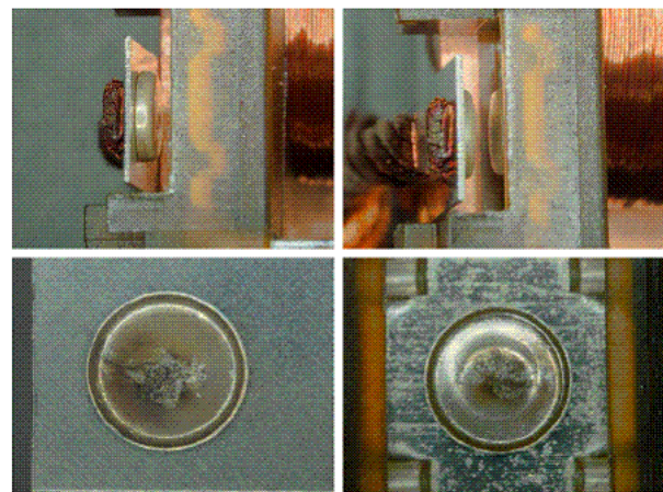
Figure 5. Contacts with minor marks.
