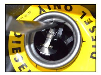
Using needle nose pliers, pull the spring loaded flap insert out of the fuel filler area <as shown>.
