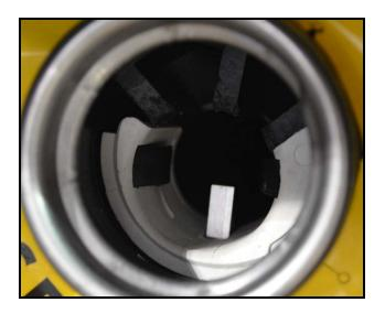
Tip: The fuel filler lockout mechanism is fully seated into position when it bottoms out against the fuel filler neck <as shown>.
