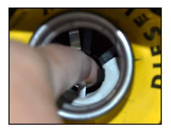
Using your finger <as shown> pull the fuel filler lockout mechanism toward you approximately 5mm until it stops.
