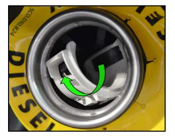
Reinsert the fuel filler lockout mechanism <as shown> and rotate from right-to-left <arrow> to seat properly into position.
