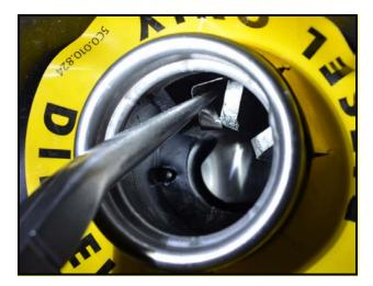
Using needle nose pliers, push the spring loaded flap insert retaining tang inward and downward until it becomes loose <as shown>.
