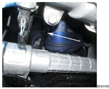
Install the new brace on 2006-2007 model year vehicles, GM P/N 12617642, using a bolt, GM P/N11570734, to attach the brace to the exhaust manifold/converter. Tighten the bolt to 58 Nm (43 lb ft).
