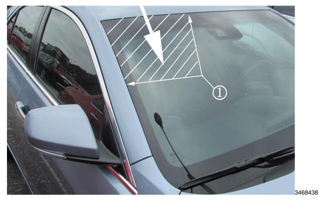
1. Perform a windshield water leak test on the passenger side of the windshield in the A-pillar area of the windshield using a water hose without the nozzle attached. Refer to photograph to view where to apply water (1).
