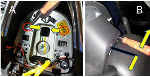
Front side of steering wheel shown in portion "A" of illustration.. Insert screw driver through the rear left and right side of the the steering wheel as shown in portion B of illustration.
