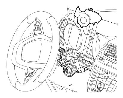
14. Install ignition lock cylinder opening cover. Refer to *Ignition Lock Cylinder Opening Cover Replacement*.
